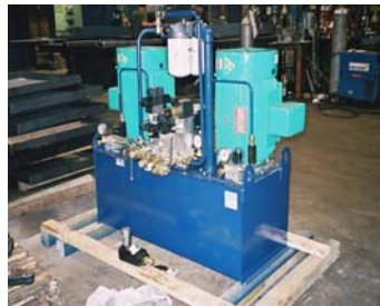
Custom power packs w/ multi functional controls
