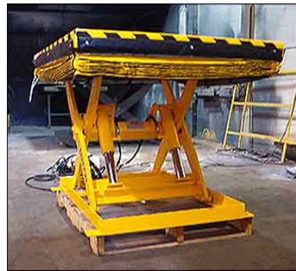
SLS w/ safety enclosure & painted safety yellow
