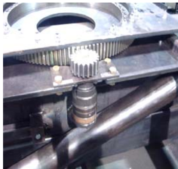
Slewing ring bearing & pinion gear drive
