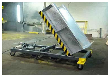
Portable tilter w/ custom galvanized platform
